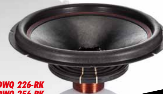
DWQ 256 380 mm or 15", 1+1 Ohm 1200W RMS, 2400W peak 4800W short burp 3" Voice coil 76mm or 3" Magnet 180 Oz
