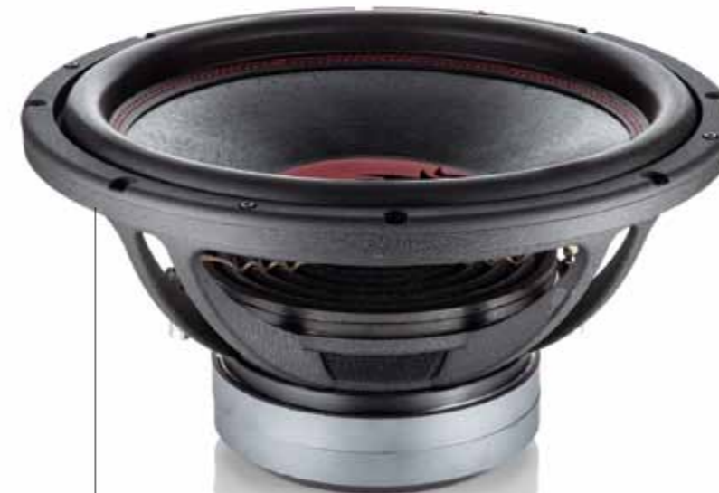
DWQ 256 380 mm or 15", 1+1 Ohm 1200W RMS, 2400W peak 4800W short burp 3" Voice coil 76mm or 3" Magnet 180 Oz
